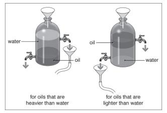
Figure 1. Florentine flasks, used to separate aqueous and oil phases.
