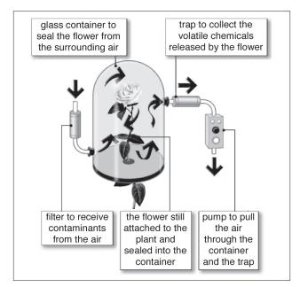
Figure 4. Headspace equipment. The volatile molecules released by the flower are swept into the trap in the stream of air. The air passes through the trap but the volatile molecules are retained. After several hours of sampling the trap is removed and taken back to the lab for analysis.
