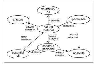
Figure 2. Extraction techniques: processes are written over the arrows and technical names for the products are circled.
