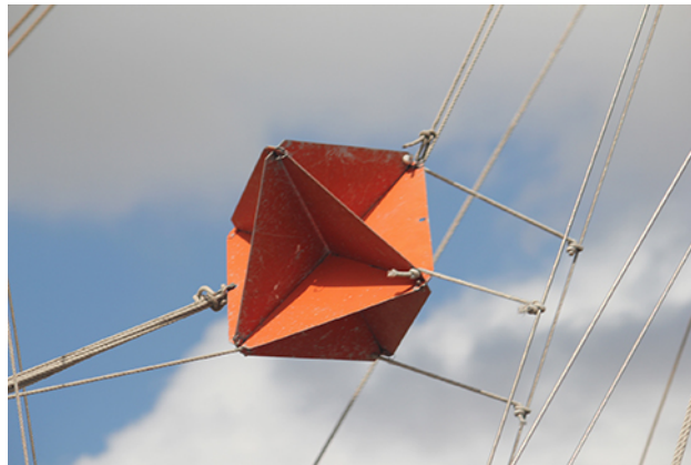
Figure 30.11 A radar reflector hoisted on a sailboat is a type of corner reflector. (credit: Tim Sheerman-Chase)
