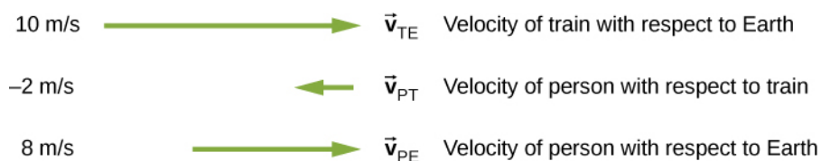
Figure 6.24 Velocity vectors of the train with respect to Earth, person with respect to the train, and person with respect to Earth.
