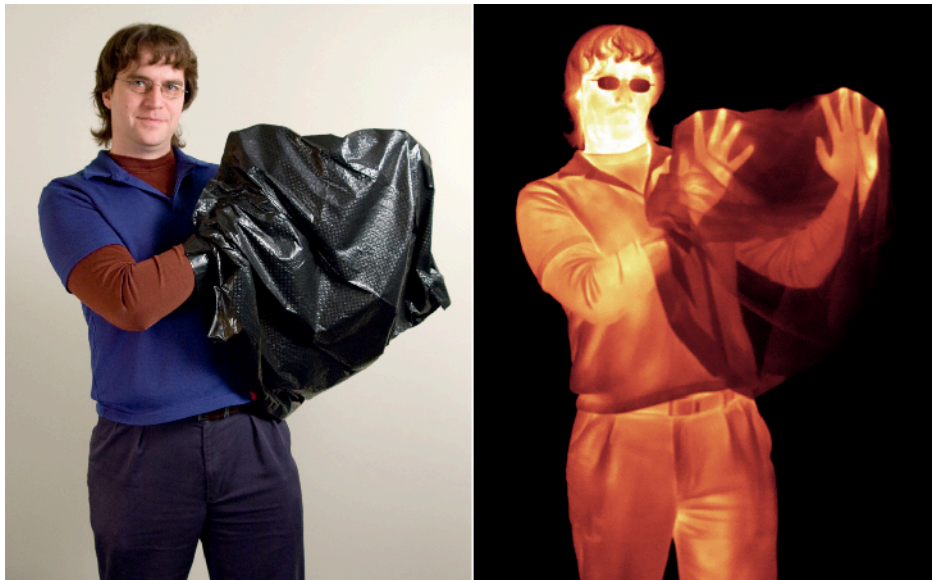
Figure 34.15 Infrared waves can penetrate places in the universe from which light is blocked, as shown in this infrared image where the plastic bag blocks visible light but not infrared. (credit: NASA/JPL-Caltech/R. Hurt (SSC))
