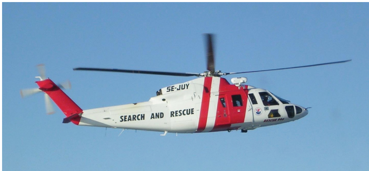
Figure 12.1 A helicopter has its main lift blades rotating to keep the aircraft airborne. Due to conservation of angular momentum, the body of the helicopter would want to rotate in the opposite sense to the blades, if it were not for the small rotor on the tail of the aircraft, which provides thrust to stabilize it.
